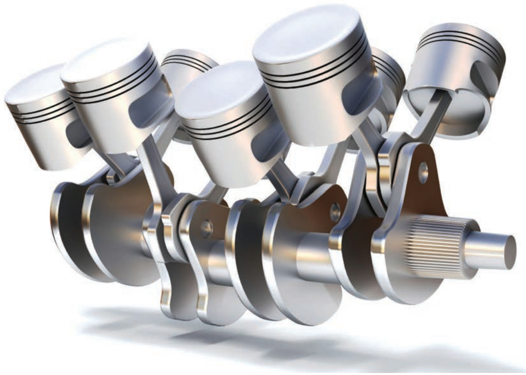
Fig 2. Piston and Connecting Rod Assembly
