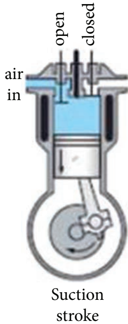
Figure 5.7.1(a) Suction Stroke
