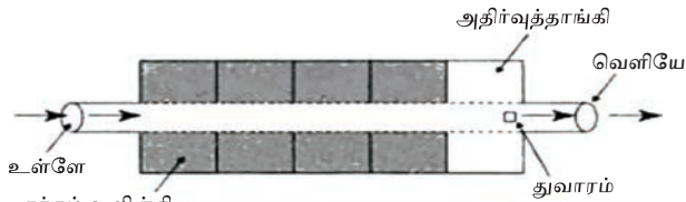
Combined resonance and absorber type muffler: 1. Inlet; 2. Noise absorbant; 3. Access port; 4. Outlet; 5. Resonant
