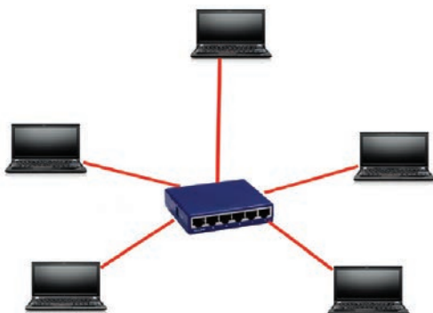
Figure 10.9: A star topology having five systems connected to a hub
