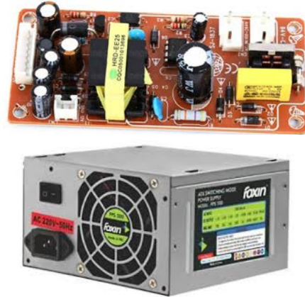
Figure 9.13 : Switched Mode Power supply
