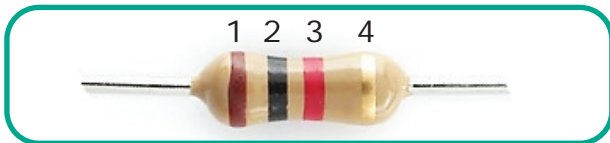
Figure 1.30 Color coding in a resistor
