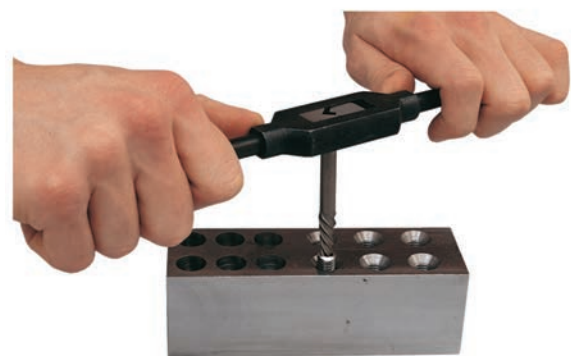
Figure 14 Type of Tap and working on Tap
