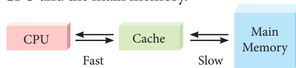
Figure 3.8 Cache Memory Arrangement
