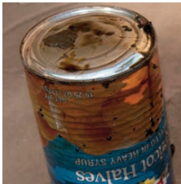
▲ Plate 8.11 Sign of Leakage
