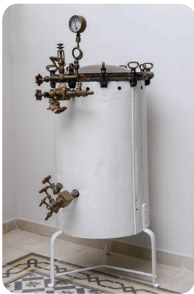
Figure 4.2: (a) Laboratory autoclave (b) Components of autoclave
