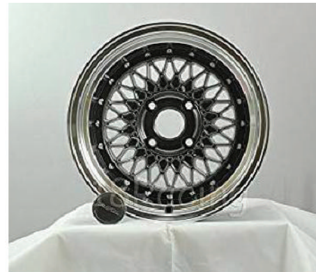
Figure 5.3.2 Structure of a Spoke / Wired Wheel
