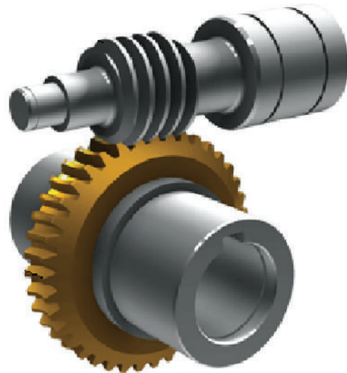
Figure 4.10.4 Worm and worm wheel arrangement
