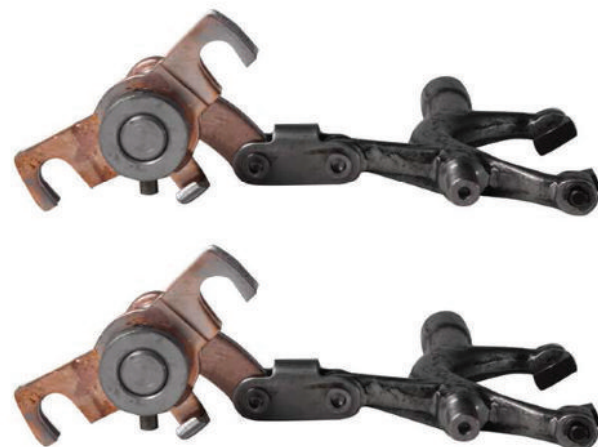
Figure 3.9.7 Gear selector mechanism
