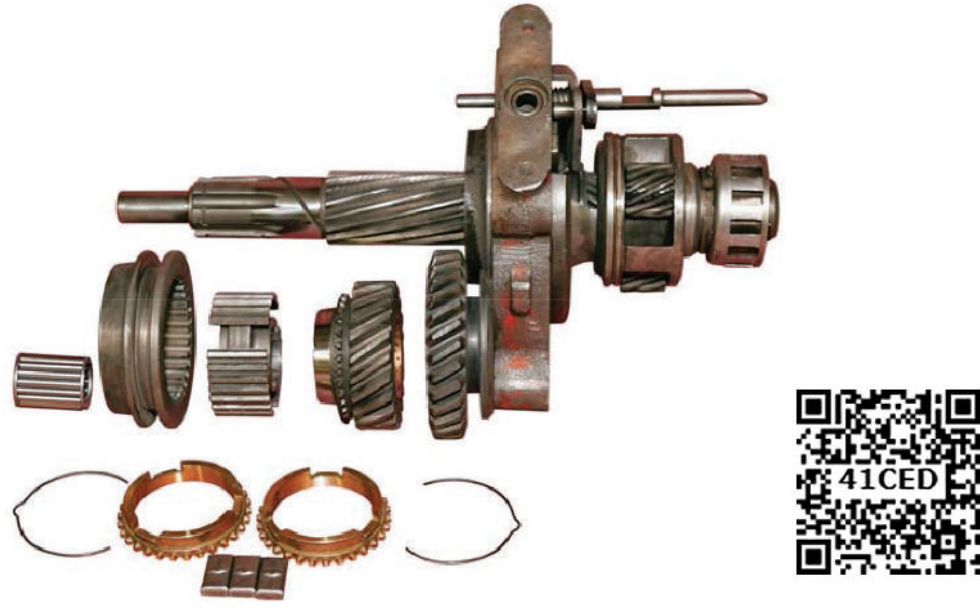
Figure 3.11.2 Important parts of a transfer case
