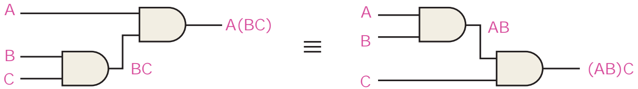
FIGURE 1.17 Associate law of three variables using AND gates
